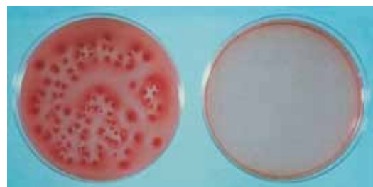
Escherichia coli bacterial colonies in contact with copper before and after 24 hours.
