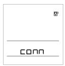
During initial operation, room unit address is set automatically. If one room unit is connected, it acquires address 1. If an additional room unit is connected, it acquires address 2. If two room units are connected simultaneously, address has to be confirmed or set on one of them, and the other room unit automatically acquires the remaining address. By factory settings, room unit 1 affects the first, and room unit 2 affects the second heating circuit.
