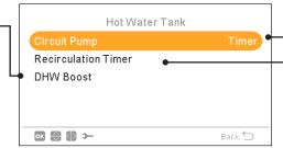
Circuit Pump: By using this output, user can heat all the water inside DHW piping system. Output must be configured at the I/O and sensors menu. (see section "7.13.4.10 Inputs, Outputs and Sensors configuration")
