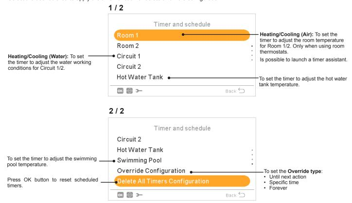
When a timer is being switched on, if that zone is stopped, it will request to switch on the zone or not.
