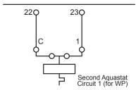
In case of YUTAKI S COMBI UK model, Domestic Hot water tank security thermostat its connected to terminals 22&23 and this funcion is not available for circuit 1.
