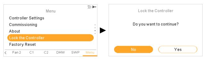
When the controller is locked the lock icon appears insted the icon menu.
