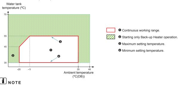
In case of heating up the DHW tank with an outdoor ambient temperature lower than -5 °C and without using the DHW electrical heater, the setting temperature must not exceed the maximum value in the specified continuous working range.
