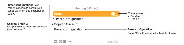
Pressing the OK button with "Timer Configuration" being selected displays the detailed schedule screen. The active schedule timers are shown in a weekly calendar.
