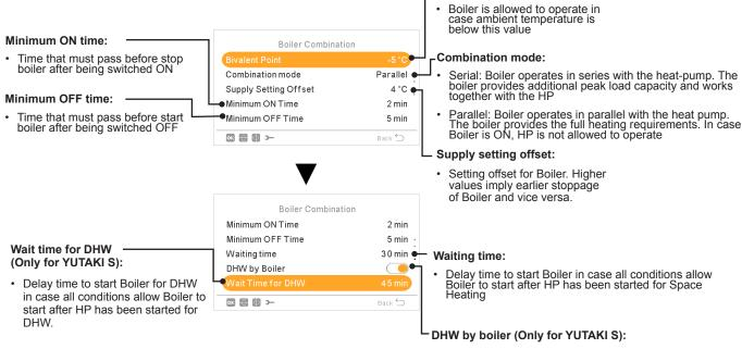
· Control to allow heat DHW by means Boiler
