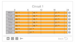
Up to six timer events can be defined for each weekday, and these can be used for turning the operation ON or OFF or to change the setting temperature. Pressing the OK key with one of the weekdays being selected in the weekly calendar screen displays the detailed schedule for the weekday.
